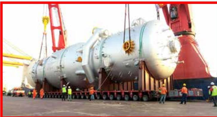
All the cargoes were handled using Megalift's Goldhofer hydraulic multi-axle modular trailers that can meet all transportation requirements of the industry and at the same time, reducing road damages and enhance safety for all road users.
