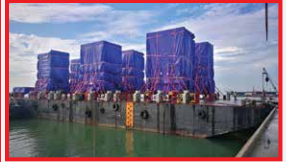
Cargo: Condenser Lower Shell Units Dimension: L7.00 m x W5.30 m x H9.60 m Weight: 75 tons each
