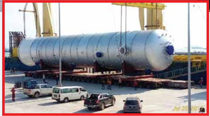
Cargo: CO2 Absorber Dimension: L44.00 m x W8.65 m x H8.55 m Weight: 471 tons
