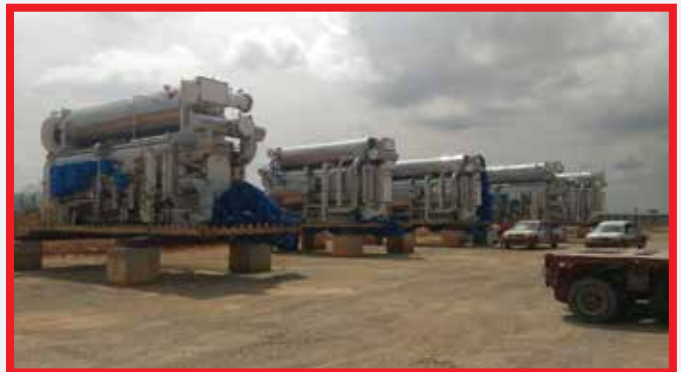
Cargo: Chiller Dimension: L11.00 m x W3.90 m x H5.00 m Weight: 53 tons each
