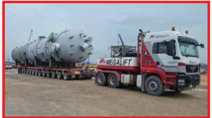
Dimension: L26.65 m x W4.64 m x H4.59 m Weight: 110.5 tons
