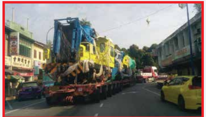
Cargo: On Truck Turnout Tamping Machine Dimension: L21.70 m x W2.78 m x H 3.92 m Weight: 75 tons
