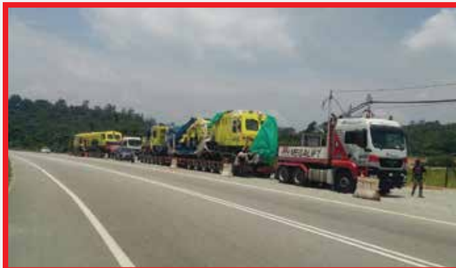
Cargo: Ballast Cleaning Machine Dimension: L25.23 m x W2.78 m x H3.92 m Weight: 77 tons
