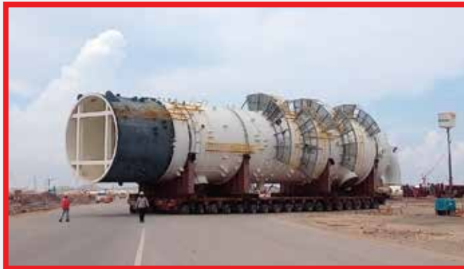
Dimension: L40.89 m x W9.93 m x H9.68 m Weight: 230 tons
