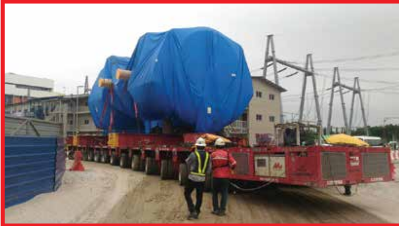
Cargo: Generator Stator Dimension: L10.95 m x W6.80 m x H5.47 m Weight: 462 tons
