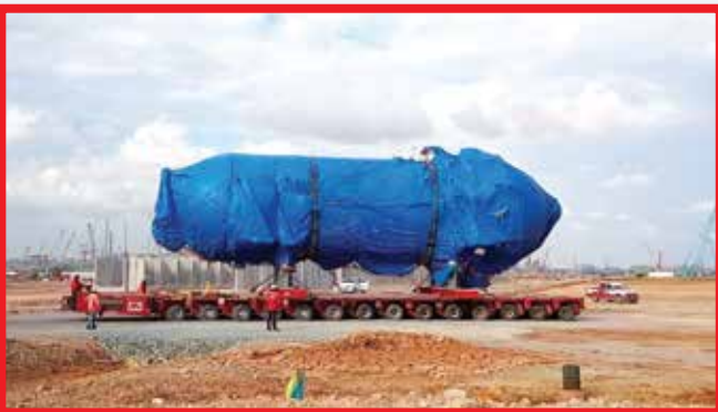
Cargo: HP Steam Drum Dimension: L20.80 m x W5.45 m x H7.35 m Weight: 262.40 tons
