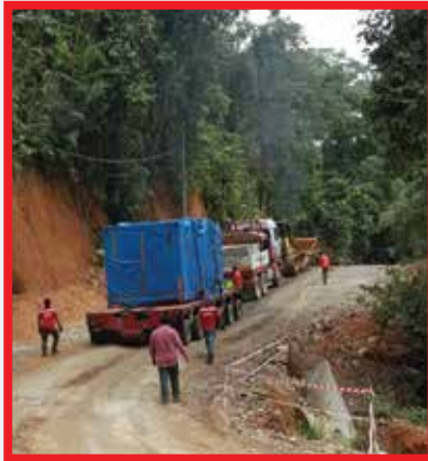
Cargo: Generator Dimension: L5.60 m x W2.40 m x H2.45 m Weight: 28 tons
