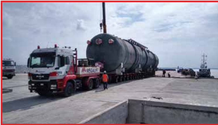
Cargo: Deaerator Dimension: L34.00 m x W5.20 m x H5.70 m Weight: 225 tons
