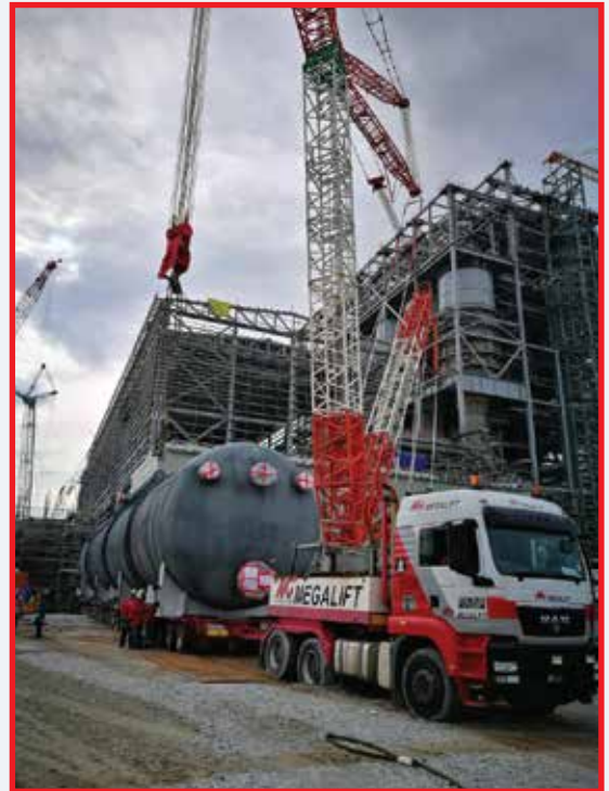
Cargo: Deaerator Dimension: L34.00 m x W5.20 m x H5.70 m Weight: 225 tons
