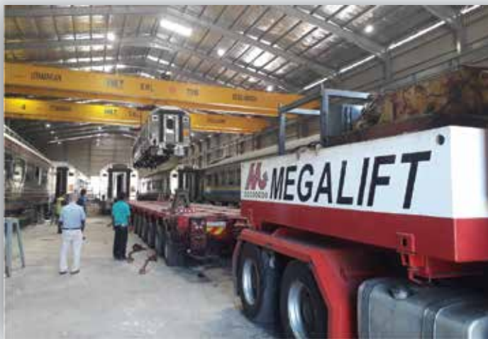
Scope: Transport Cargo: Coaches (5 units) Dimension: L21.00 m x W2.43 m x H2.74 m Weight: 25 ton
