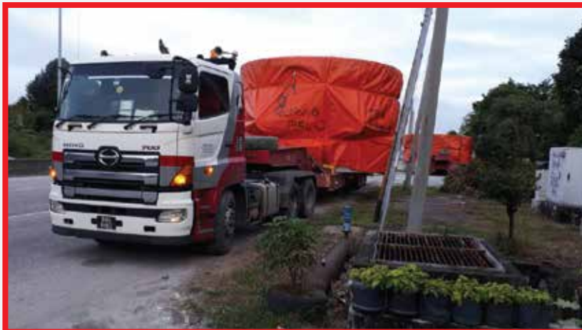
Dimension: L6.80 m x W6.63 m x H3.00 m Weight: 26.60 ton Scope: Transportation from Jalan Meru to Westports
