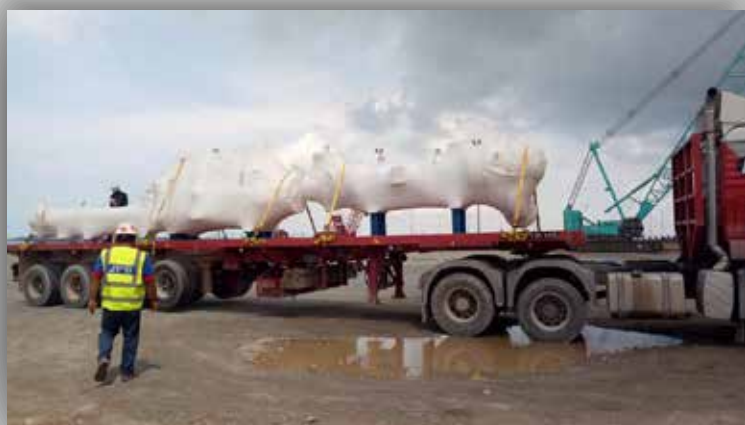
Cargo: Gas Compressor Unit Dimension: L9.70 m x W4.90 m x H6.40 m Weight: 44.15 ton
