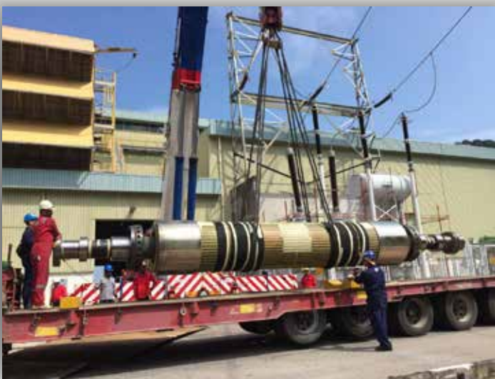
Scope: Heavy lifting Cargo: Rotor Dimension: L10.25 m x W1.20 m x H1.20 m Weight: 41.50 ton
