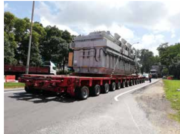
Transportation of Generator Stator | L11.90 m x W4.86 m x H4.92 m | 453 ton
