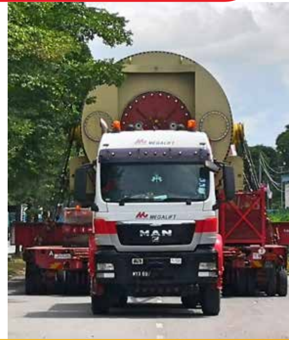
Transportation of Generator Stator | L11.90 m x W4.86 m x H4.92 m | 453 ton
