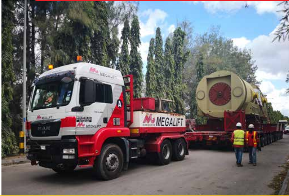
Transportation of Generator Stator | L11.90 m x W4.86 m x H4.92 m | 453 ton
