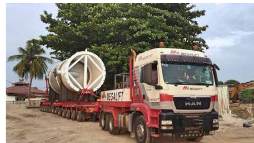
Reactor Feed/Effluent Exchange L10.89 m x W6.05 m x H7.57 m 235.9 ton
