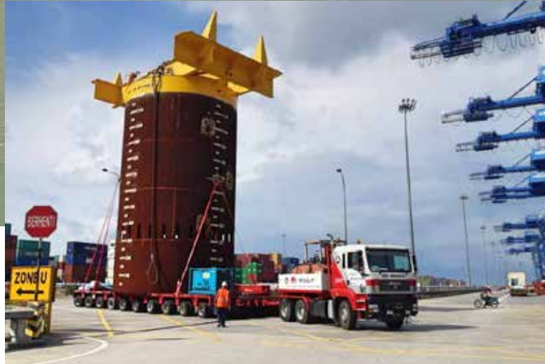
Cargo 1: Hub Manifold Suction Anchor Dimension: L7.50 m x W7.50 m x H16.40 m Weight: 96 ton
