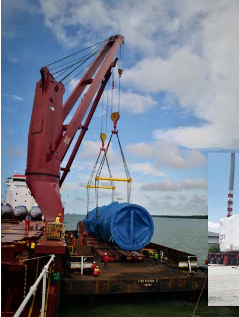
Cargo: HDS Reactor Dimension: L38.52 m x W7.20 m x H7.25 m Weight: 466 ton
