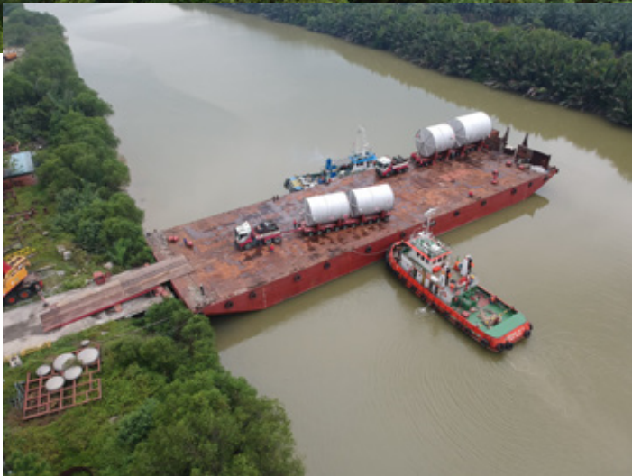
Cargo: Product Silo Dimension: L22.68 m x W7.12 m x H7.31 m Weight: 42 ton
