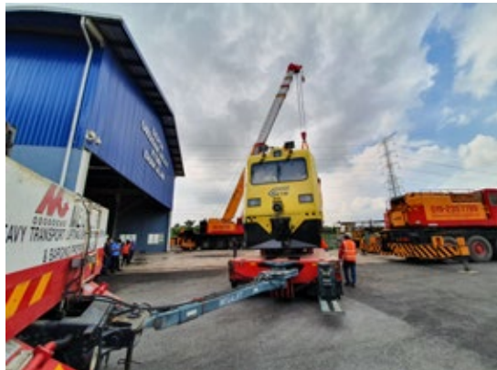
Cargo: Machine 7084 Train Set Dimension: L21.26 m x W2.91 m x H4.03 m Weight: 59 ton
